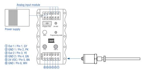
Fig. 24: Connecting sensor with cabinet programmer
