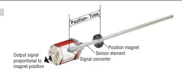
Fig. 1: Principle of operation:
