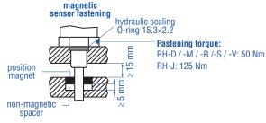
Fig. 15: Installation with magnetizable material
