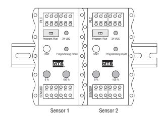
Fig. 23: Dimensions: 10 × 55 × 31 mm; Material: Aluminum, side caps PA 6.6 FR; Connection: Spring terminals, max. 1.5 mm<sup>2</sup>; Protection: IP20
