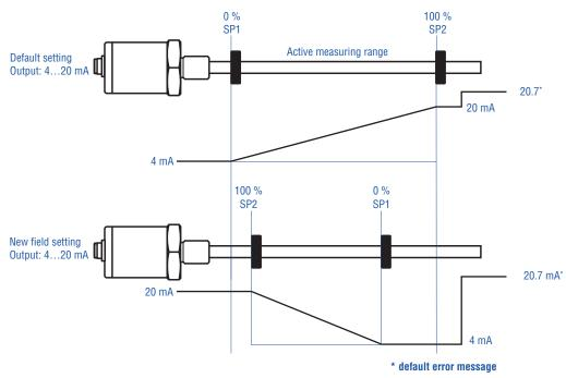
Fig. 32: Start and end point, set the direction
