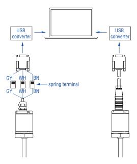
Fig. 26: Programmer connectiong (left: with spring terminal, right: with cable)
