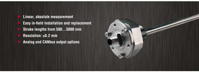
Designed for use with hydraulic cylinders in mobile applications, the externally threaded Flexible MH sensor features an innovative two-part design. This design allows users to separate the flexible sensing element and electronics from the housing without opening the hydraulic system.
