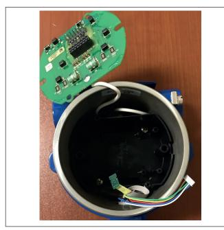
Fig. 6: Sensing element Disconnected
