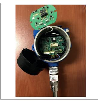
Fig. 4: Top board removed
