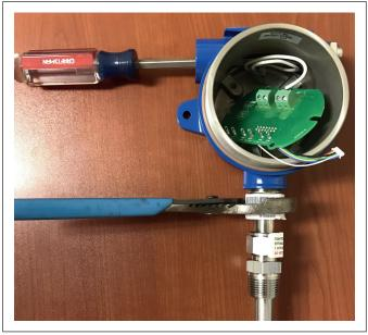
Fig. 8: Housing removal
