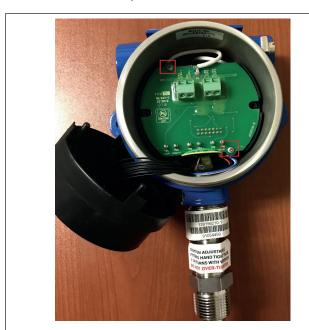
Fig. 3: Screw removal
