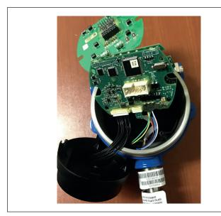
Fig. 12: All boards removed
