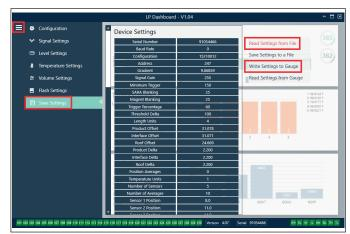
Fig. 6: LP Dashboard - Save Settings - Write to Gauge
