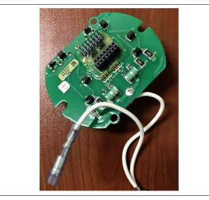
Fig. 15: Ground Lug Removed
