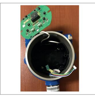
Fig. 13: Sensing Element disconnected
