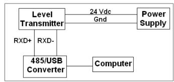
Fig. 2: Connection diagram for Modbus or DDA
