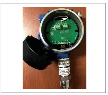
Fig. 9: Display Removed
