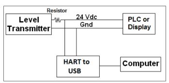
Fig. 1: Connection diagram for HART® outputs
