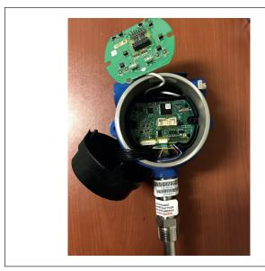
Fig. 11: Top Board Removed
